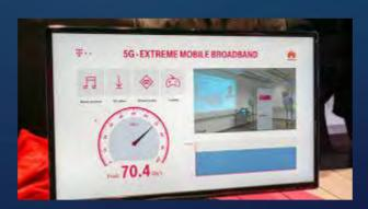
World Record: 70 Gbps on the 73 GHz millimeter wave band
