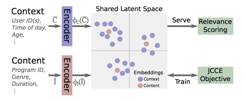
Two nonlinear encoder networks consisting of three fully connected layers each. The first two layers are each defined to have 250 rectified linear units (ReLUs), and the last layer is a linear transformation with 50 units.
