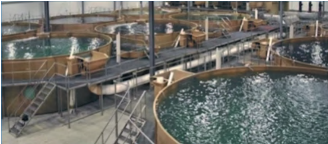
Fig. 1.15. Indoor recirculating aquaculture system
