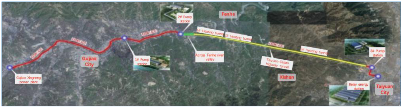
Fig. 2.14. General layout of the main heating pipeline from the Gujiao power plant to Taiyuan. Constructed from an aerial photograph from Google Earth
